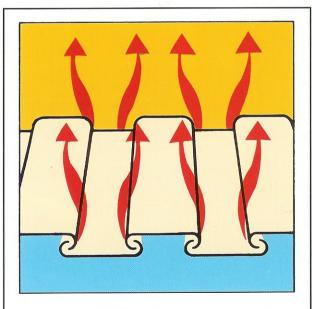
Aurora Awnings have a natural venting action to prevent the build up of hot air against windows. The unique "pan and cover" construction helps keep rain, snow and debris from penetrating, without trapping heated air underneath. It also allows a soft "halo light" to filter into your home instead of dark shadows associated with other awnings. And, unlike fabric awnings, Aurora Awnings won't stretch or tear, and they don't need to be taken down in winter.
